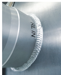
Uniform, full, and aesthetically shaped fish scale welds
